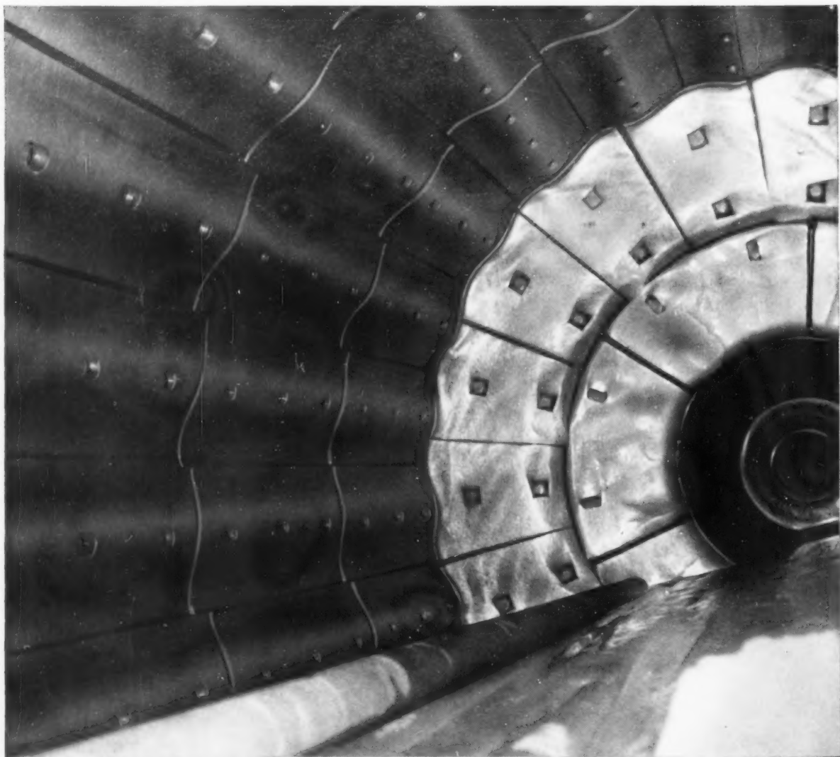
The Ni-Hard iron liners in this rod mill have saved over $16,000. Cost per ton of ore dropped to 0.89 cents, compared with 2.50 cents per ton for manganese steel liners formerly used.
